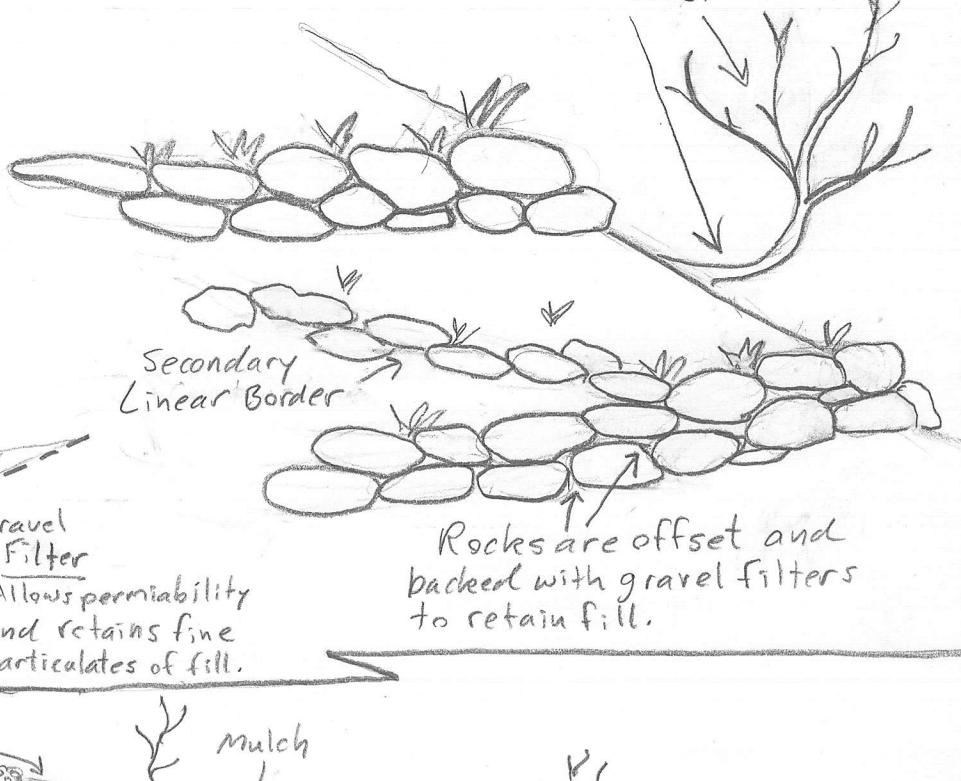
Dry laid rocks are angled in towards slope to increase stability and retain fill. This accounts for both downhill slump and gravity.
